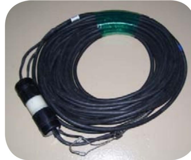
Fly cable for Chain Master hoists is a 14-4 cable with a hubbell male connector HBL2421, and a hubbell female connector HBL2423.
